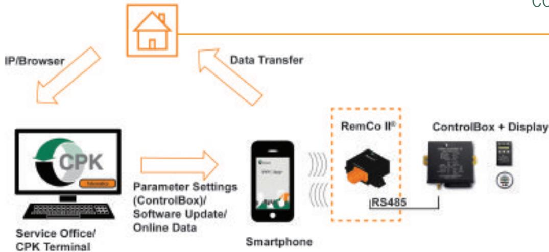
The RemCo II remote control module by CPK works in conjunction with the Dyntest emissions control system. The collected, encrypted data are transferred via Bluetooth to a smartphone, where a special app allows users to transfer the data into a dedicated web portal for analysis.
